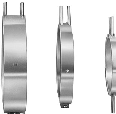
**Maxiband MXC Bands** are made for cooling only and are available in five standard widths: 3/4", 1-1/2", 2-1/2", 3", and 4". For 3/4" and 1-1/2" wide MXC bands the ends of the stainless steel cooling tubes exit 180° apart. Complete Maxiband specifications can be found on page 1-81.
