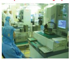
**Quality Control using Automated Test Equipment in a Clean Room Environment**
